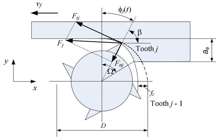
Fig. 1. Representation of cutting forces in milling (up milling).
