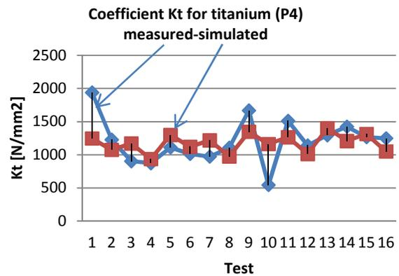
Fig. 9. Variation diagram of coefficient  $K_n$  (given by (13)) and modeled for titanium.
