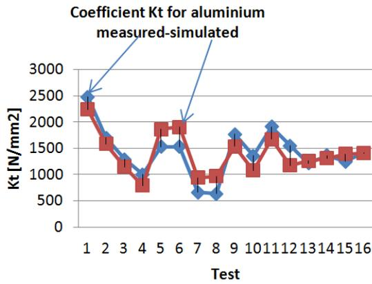
Fig. 12. Variation diagram of coefficient  $K_t$  (given by (13)) and modeled for Al 7178.
