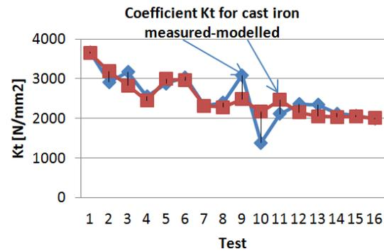
Fig. 10. Variation diagram of coefficient  $K_t$  (given by (13)) and modeled for cast iron.
