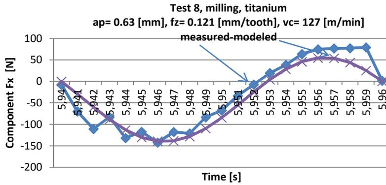
Fig. 16. Comparison diagrams of component  $F_x$  (measured-modeled) for titanium.
