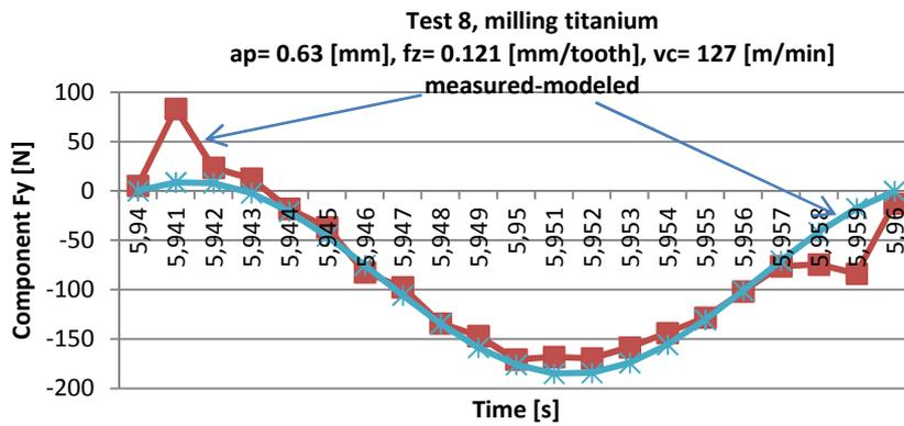
Fig. 17. Comparison diagrams of component  $F_y$  (measured-modeled) for titanium.
