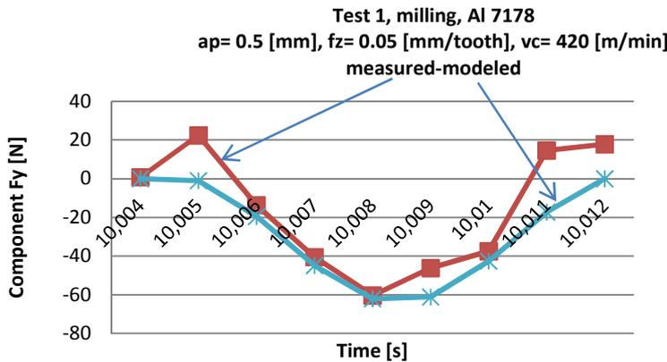
Fig. 19. Comparison diagrams of component  $F_y$  (measured-modeled) for Al 7178.
