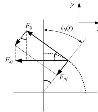
Fig. 2. The scheme of the forces for determining component  $F_x$  of the cutting force in milling.
