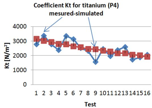
Fig. 8. Variation diagram of coefficient  $K_t$  (given by (13)) and simulated for titanium.
