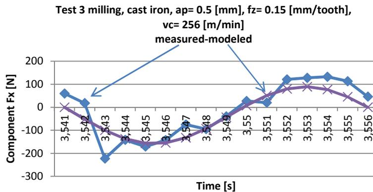
Fig. 14. Comparison diagrams of component  $F_x$  (measured-modeled) for cast iron.
