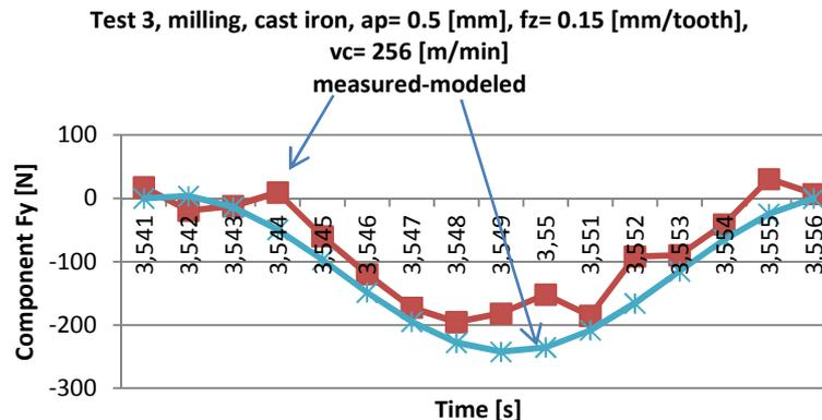
Fig. 15. Comparison diagrams of component  $F_y$  (measured-modeled) for cast iron.
