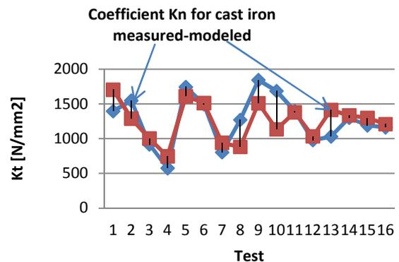
Fig. 11. Variation diagram of coefficient  $K_n$  (given by (13)) and modeled for cast iron.
