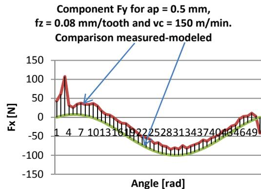
Fig. 5. Comparison diagrams of component  $F_y$  (measured-simulated).
