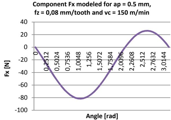
Fig. 3. Change in component  $F_x$  (force modeled, OLC 45).
