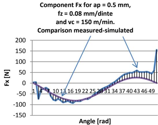
Fig. 4. Comparison diagrams of component  $F_x$  (measured-simulated).
