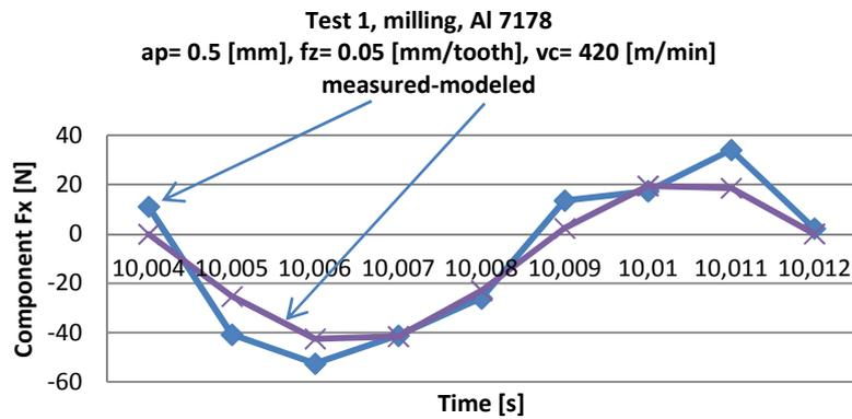
Fig. 18. Comparison diagrams of component  $F_x$  (measured-modeled) for cast iron Al 7178.
