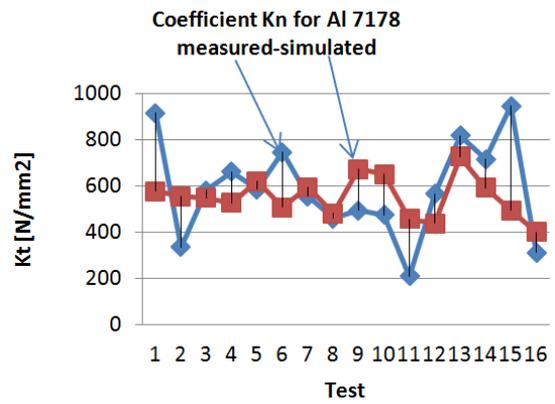
Fig. 13. Variation diagram of coefficient  $K_n$  (given by (13)) and modeled for Al 7178.
