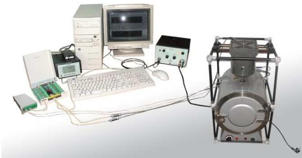
**Fig. 1.** Experimental stand used for real-time monitoring of the processing of composites with polymeric matrix materials.
