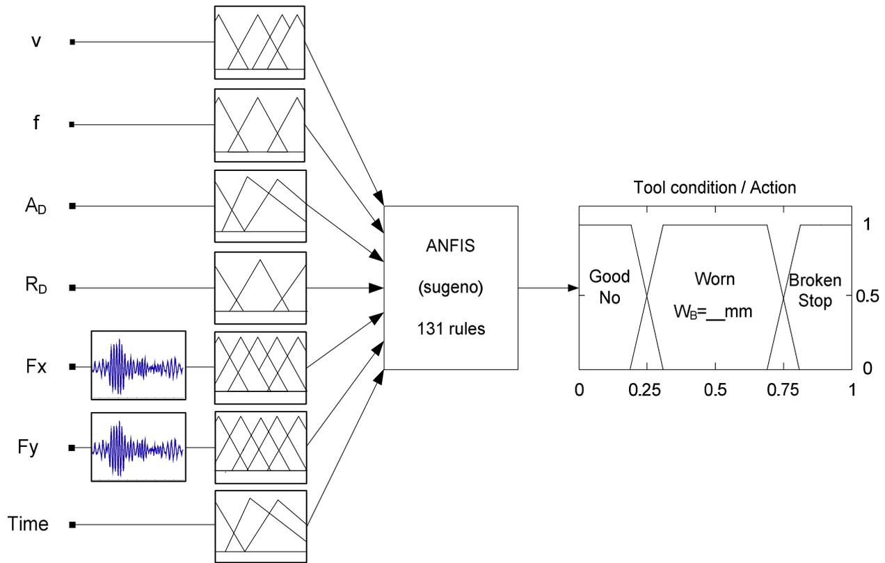
Fig. 2. ANFIS tool condition and wear estimator.
