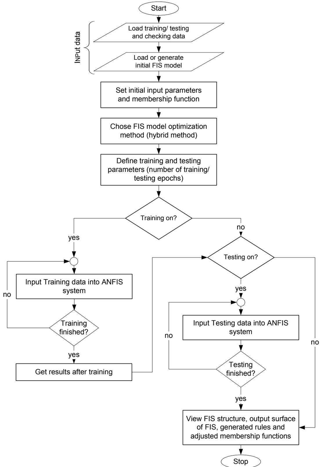
Fig. 2. ANFIS tool condition and wear estimator.
