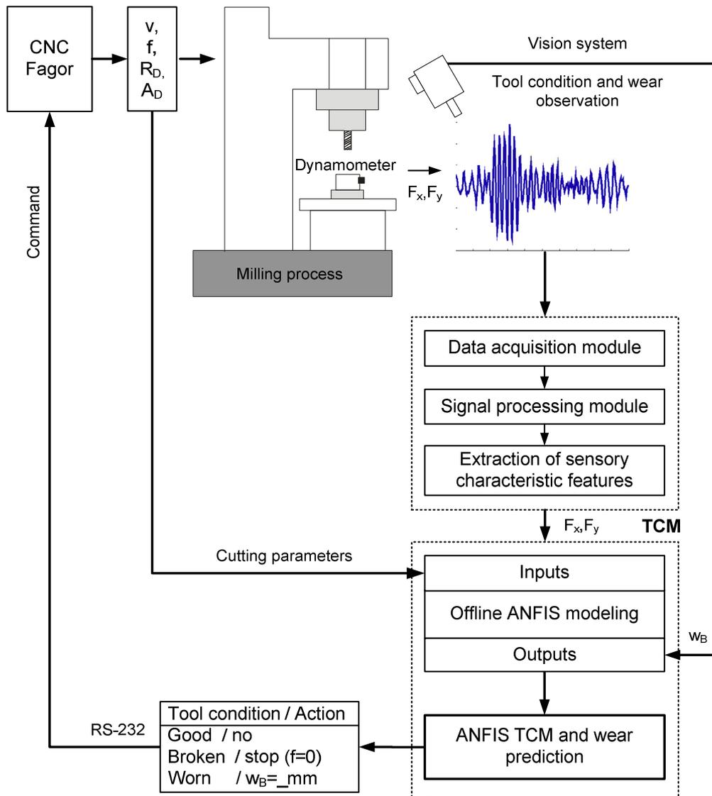
Fig. 1. Architecture of tool condition monitoring system.
