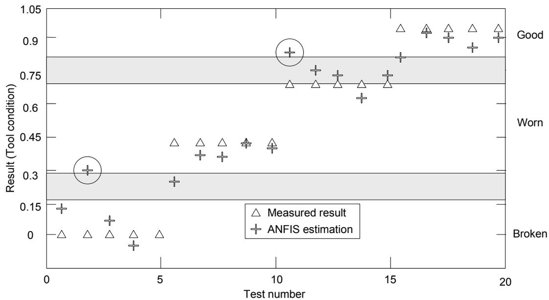
Fig. 3. ANFIS output of tool condition.
